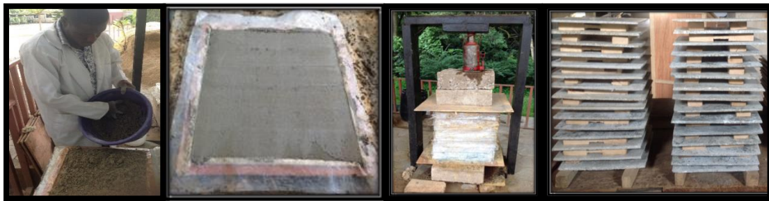
Plate 4: Formation Process of the Composite Board (spreading, moulding, cold pressing and 28 days curing/air-drying)
