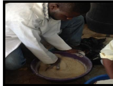
Plate 2: Homogenous mixing of the materials (Sawdust, Cement and Glass Powder)
