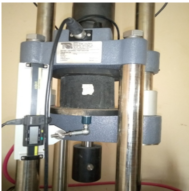
Figure 2. Test for the compressive strength of the briquette using a Universal Testing Machine
