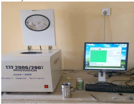
Figure 1. Test for the calorific value of the briquette using a bomb calorimeter
